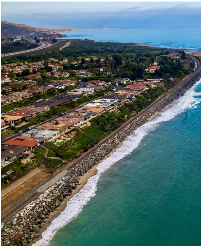
Left: Orange County Transit Authority's existing rock riprap at Cotton's Point has increased erosion and blocked lateral access to Trestles. Right: Community members came together to listen, learn, and share their vision for San Onofre's future.
