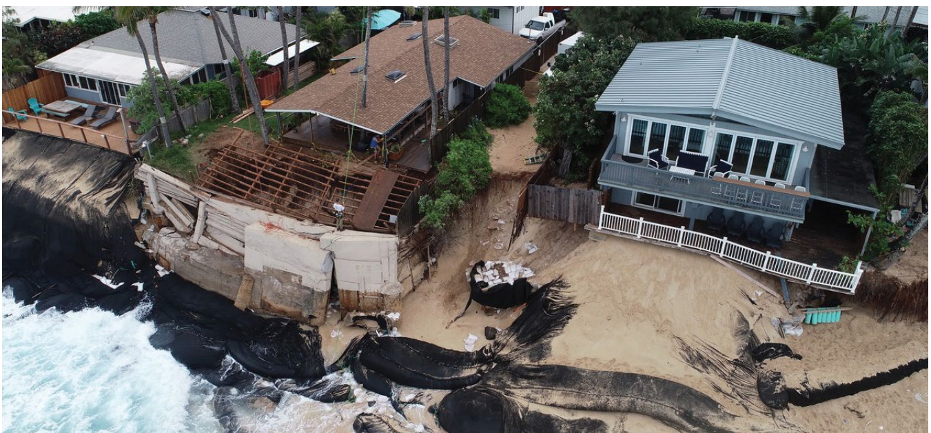
To protect their homes from the encroaching sea, homeowners resort to short-term fixes like geotextile burritos, erosion skirts, and unauthorized concrete.
